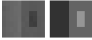
Fig. 3. Original image is in the left, and the corresponding segmented image is in the right when k = 1, \varepsilon = 5 \approx \text{Ave}(1) = 4.5630 in (11).
